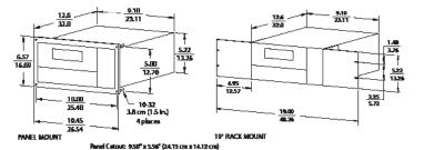
APPROX. WEIGHTS: NEMA 4 WALL/PANEL MOUNT: 28 LB / 12.7 KG 19° RACK MOUNT: 14 LB / 6.35 KG PANEL MOUNT: 14 LB / 6.35 KG
