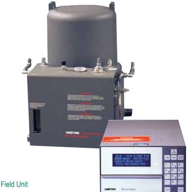
The field unit is explosion-proof and is certified to comply with numerous international standards. It contains a sample cell, switching valves and associated electronic circuits mounted internally and a flowmeter, flow control valves and back pressure regulator mounted
